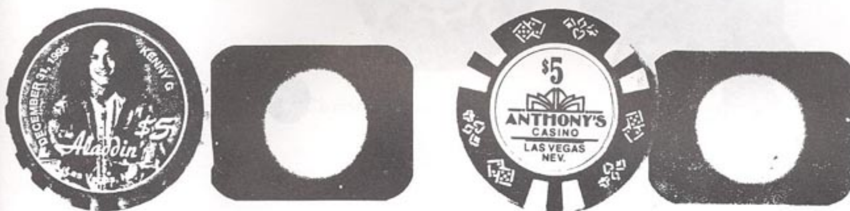
More Bud Jones injection mold chips with x-rays
